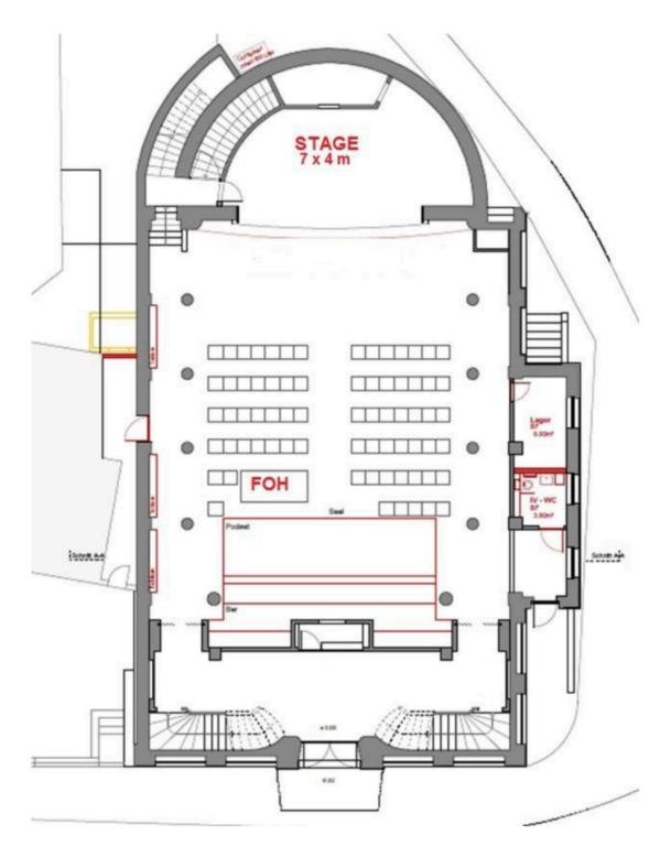
Stage: 4 x 7 meters (semi-circle Stage height: 6.2m Stage – FOH: 8.5m Room length: 13.5m Room width: 13.7m Capacity: 400
